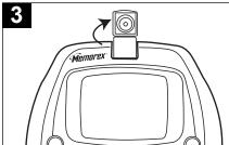
Open the camera compartment. The camera will then show the image on the built-in screen. Rotate the Camera Focus Adjusting Ring located on the outside of the lens to adjust the camera's focus.
